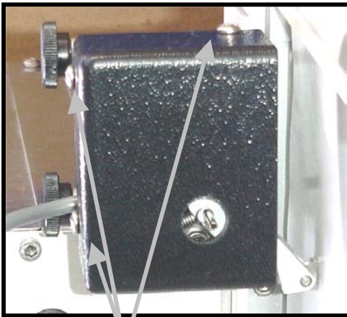
Fig 21 Remove 3 Pan head screws
