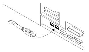
Insert USB cable into the down stream port of the PC (or) this product. Make sure that it goes all the way into the socket and is firmly connected.
