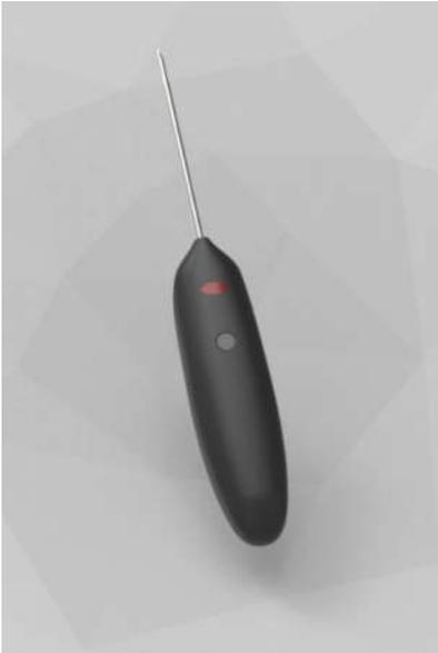
The Handheld Temperature Probe is developed to perform a manually triggered temperature measurement activity of the desired zone or touched product. By pushing the button, the probe will be activated and start the measurement. After 5 seconds of stabilized contact, the temperature figure collected will be send to the server using IEEE 802.15.4 communication protocol.
