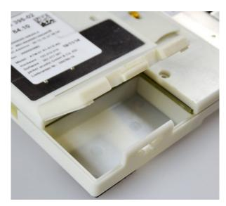
Remove the battery and replace it with a new one of the same type (BMW 9 361 678-XX).
