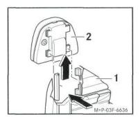
Insert the Mercedes-Benz V3 Cradle (1) into the latches on the pre-installed MHI contact plate (2), located in the center console.
