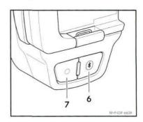
With Mercedes-Benz V3 Cradle connected to the vehicle press button (6) for approx. 2-3 seconds.
