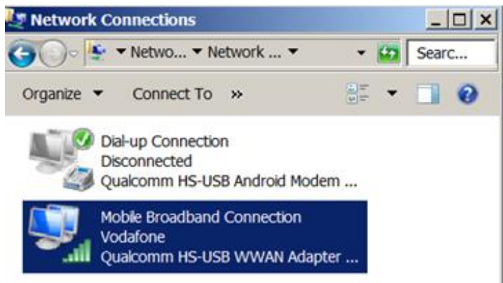
Figure 15 The USB driver provides a NIC (Network Interface Card).
