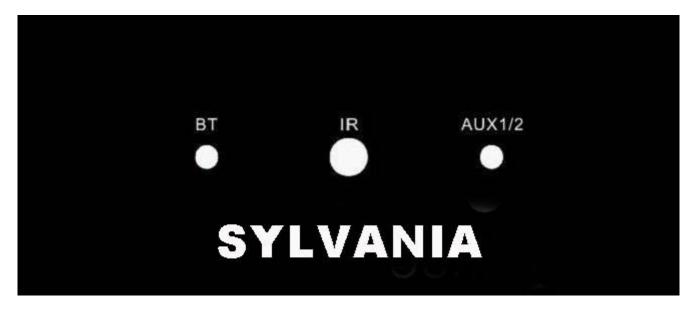
BT: The Indicator for bluetooth input status. Frequent blinks of the LED indicate a failure of the communication, while infrequent ones indicates a successful communication
