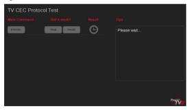
Each test is launched by selecting an item in the 'Main Command' column and pressing ok , the result of the test is registered by selecting the appropriate button under the "Did it Work" column.
