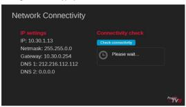
The information window will either display "network successfully configured" with the next button selected, or a 'connectivity fail' message if the OnAir SBB was unable to reach the internet, in which case all network and Common Data entered must be checked and the procedure retried. The RCU back button can be used to re-enter forms to check data. When the 'network successfully configured' message is display, skip next section and proceed directly to 'Step 6: The Wi-Fi bubble' on page 20.
