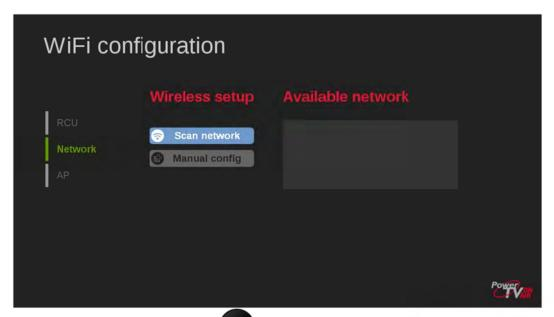
Select 'Scan network' and press to display the SSIDs of available networks.
