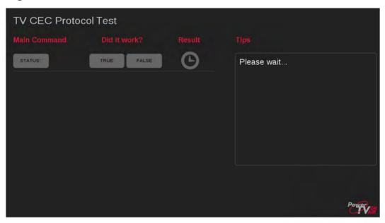
Each test is launched by selecting an item in the 'Main Command' column and pressing the result of the test is registered by selecting the appropriate button under the "Did it Work" column.
