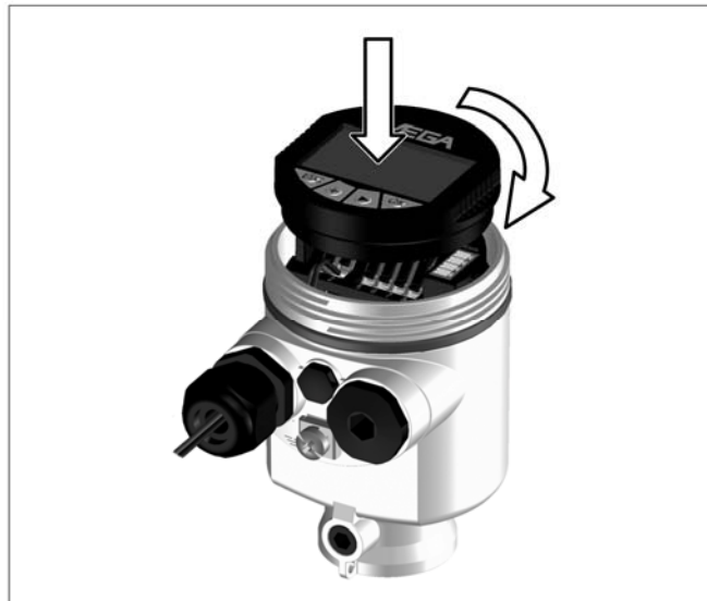
Fig. 25: Installation of the indicating and adjustment module
