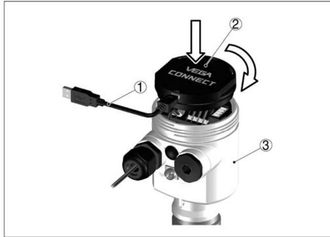
Fig. 29: Connection of the PC via VEGACONNECT directly to the sensor
