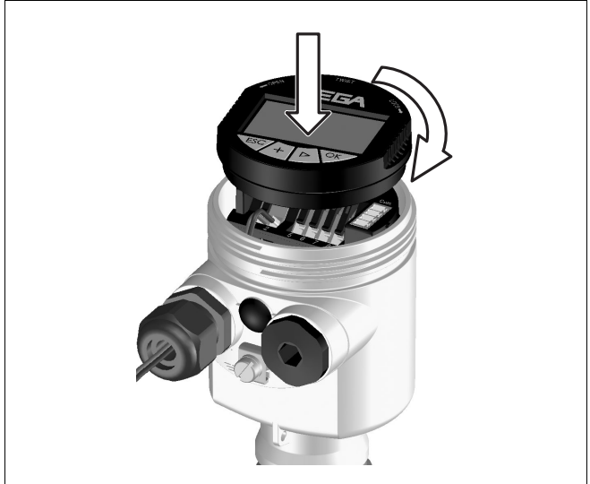
Fig. 26: Installation of PLICSCOM
