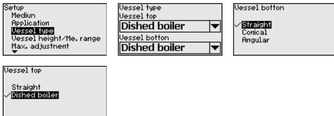
Enter the requested parameters via the appropriate keys, save your settings with [OK] and jump to the next menu item with the [ESC] and the [->] key.
