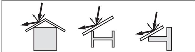
Fig. 14: Cover flat, large-area profiles with deflectors
