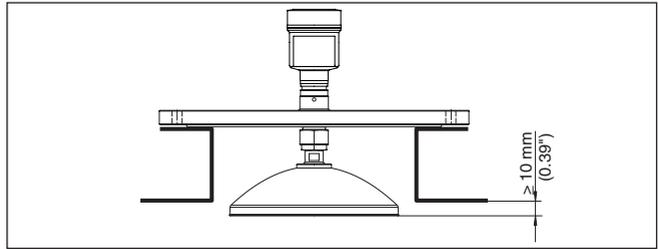
Fig. 9: Recommended socket mounting with parabolic antenna
