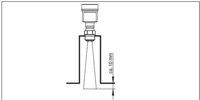
Fig. 8: Recommended socket mounting with horn antenna
