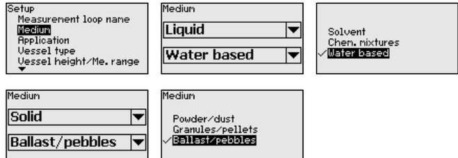
Through this selection, the sensor is adapted perfectly to the product and measurement reliability, particularly in products with poor reflective properties, is considerably increased.
