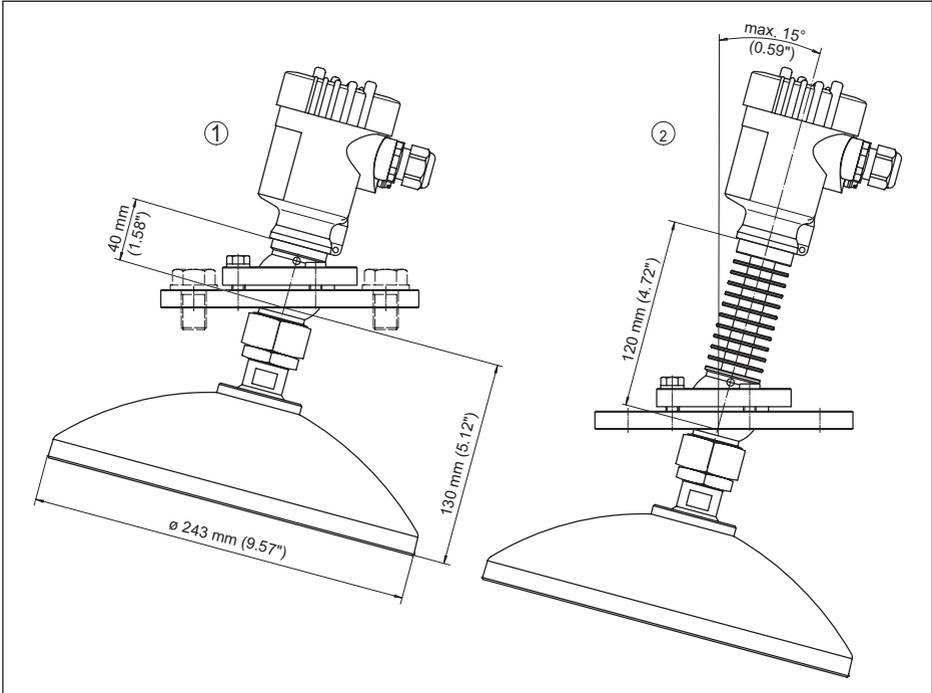
Fig. 69: VEGAPULS 62, parabolic antenna and swivelling holder
