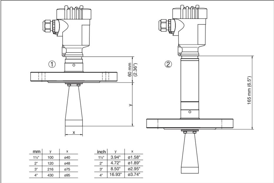
Fig. 64: VEGAPULS 62, horn antenna in flange version
