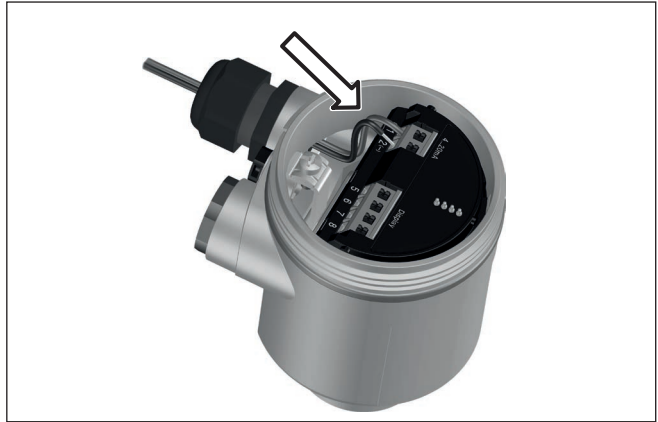
Fig. 25: Connection steps 5 and 6 - Single chamber housing
