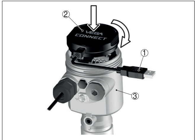
Fig. 44: Connection of the PC directly to the sensor via the interface adapter
