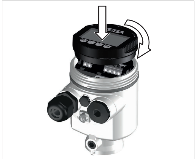
Fig. 41: Installing the display and adjustment module in the electronics compartment of the single chamber housing
