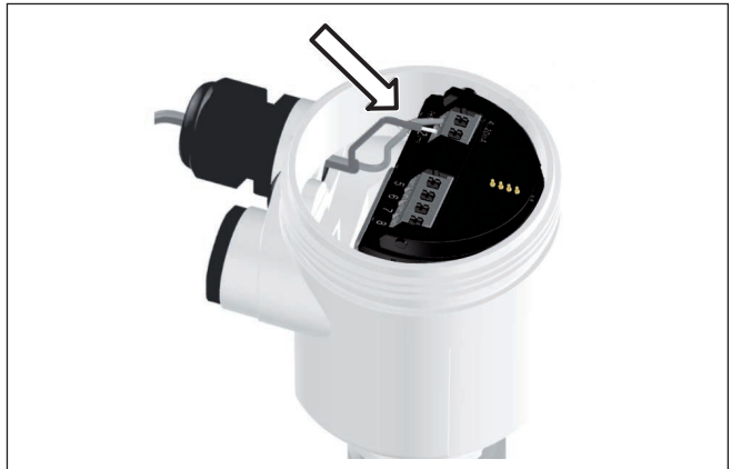
Fig. 26: Connection steps 5 and 6 - Single chamber housing
