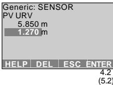
After having pressed "ENTER", press "SEND" (here in the example for the min. adjustment).
