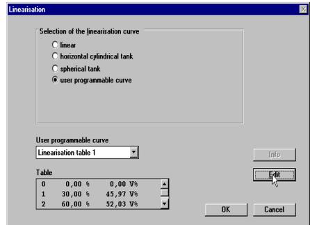
A linear correlation between product distance (in %) and filling volume (in %) has been preset. Besides the two programmed linearisation curves "*Cylindrical tank*" and "*Spherical tank*" you can also enter "*user programmable curves*". Linear means that there is a linear correlation between level and volume.
