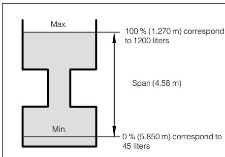
Max. 32 index markers can be entered per linearisation curve (value pairs).
