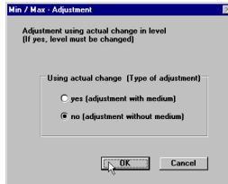
You can carry out the min./max. adjustment with medium or without medium. Generally you will carry out the adjustment without medium. When you want to carry out the adjustment with medium, you have to carry out the min. adjustment with emptied vessel and the max. adjustment with filled vessel.
