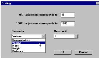
As physical quantity you can choose "dimensionless (plain numbers), volume, mass, height and distance" and assign an appropriate unit of measurement (e.g. l, hl). The sensor display then shows the measured value in the selected physical quantity and unit.
