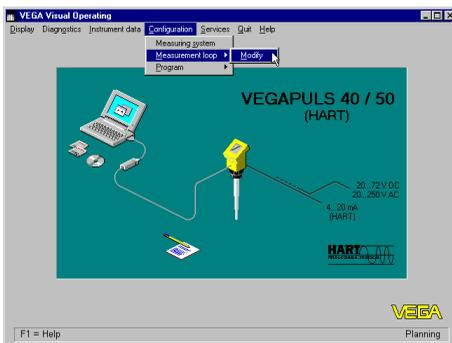
In the menu "Modify meas. loop configuration" you can give a name (e.g. vessel 10) and a description (e.g. sludge separator) to the measurement loop.
