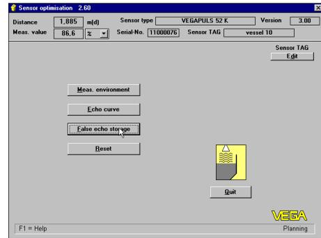
With the menu item "False echo storage" in the menu "Sensor optimisation", you can authorise the sensor to save false echoes. The sensor electronics then saves the false echoes in an internal database and assigns them a lower level of importance than the useful echo.
