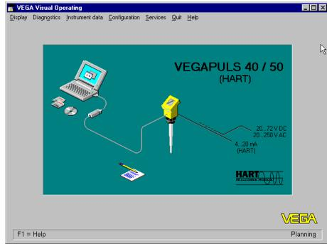
... and indicates after a few seconds if and with which sensor a connection exists.
