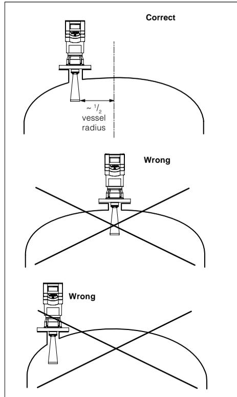
Mounting on a vessel with parabolic tank top
