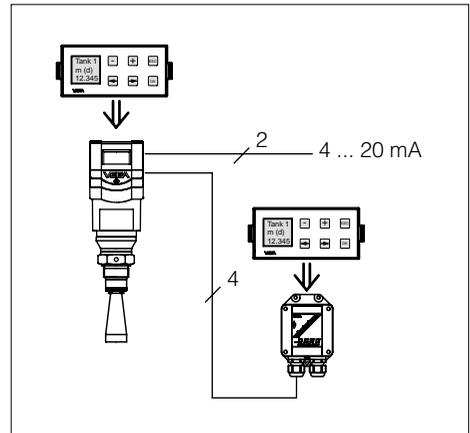
For the adjustment with adjustment module, all sensor versions (adjustment options), as with the PC and the adjustment program VVO, are available. There are some differences, however, with MINICOM. It is not possible to enter your own linearisation curve.
