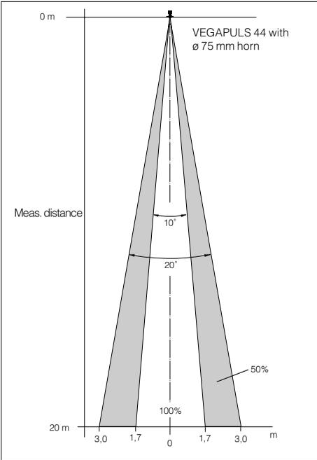
Emission cone of a DN 80 flange antenna
