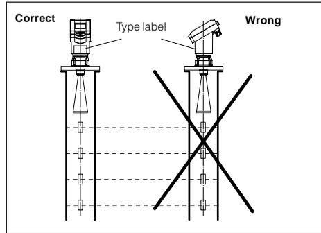
*VEGAPULS 44 on the surge pipe: The sensor type plate must be aligned with the rows of holes.*
