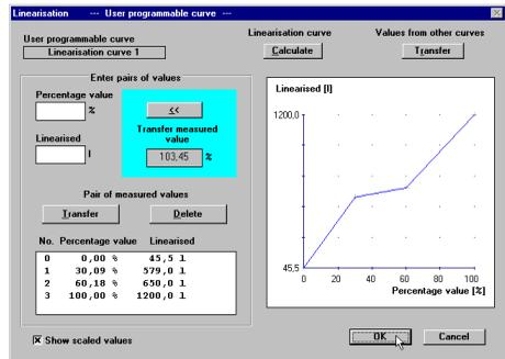
You are again in the menu window "Linearisation -- user programmable curve --". The volume percentages, with the corresponding level percentages, are shown as scaled values (liters in this example), if you have clicked in the check box in the bottom left corner of the window.
