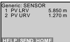
After pressing "SEND", a warning is displayed which informs you that you are about to modify the configuration, and that for safety reasons, you should switch your system over to manual operation.
