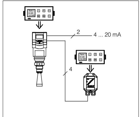
Adjustment with detachable adjustment module. The adjustment module can be plugged into the radar sensor or the external indicating instrument VEGADIS 50.
