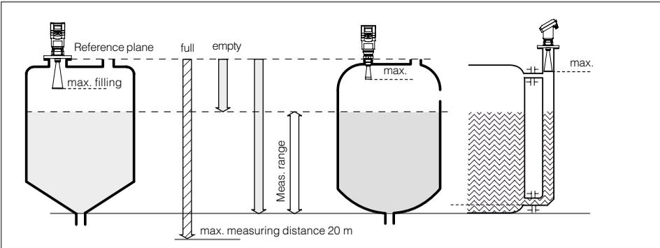
Measuring range (operating range) and max. measuring distance
