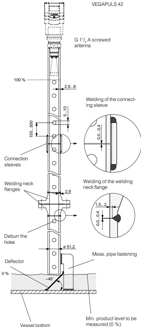
Radar sensors for measurement on surge or bypass pipes are routinely mounted in flange sizes DN 50, DN 80, DN 100 and DN 150. The radar sensor with a DN 50 flange forms a functional measuring system only in conjunction with a measuring pipe.
