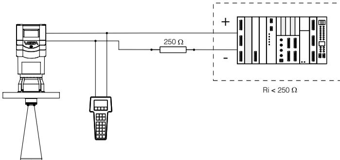
**Connection to a VEGA signal conditioning instrument**
