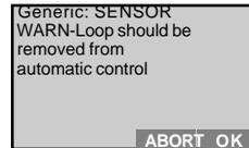
Press "OK" and the adjustment will now be transferred to the sensor. After a short time you are asked to switch your system over from manual to automatic operation. Confirm with "OK".
