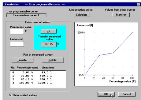
Visualised input of a vessel linearisation curve
