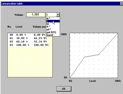
After a short calculation time, the levels as a percentage of span and the corresponding volume percentages are shown. The outputted curve shows this correlation in a diagram.
