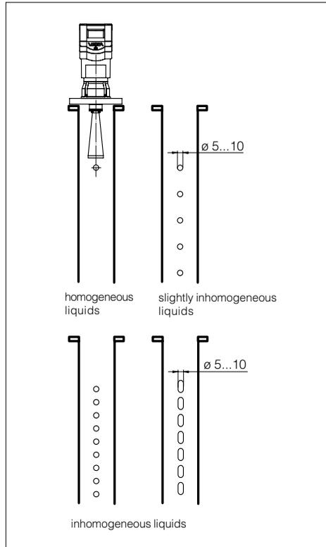
Openings in a surge pipe for mixing of inhomogeneous products
