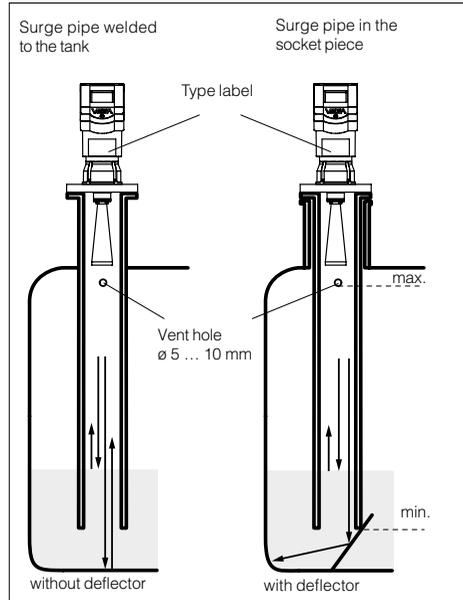
*Pipe antenna systems in the tank*
