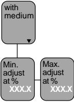
Fill the vessel e.g. to 10 % and enter 10 % in the menu "Min. adjust" with the "+" and "-" keys. Then fill the vessel, e.g. to 80 % or 100 % and enter 100 % in the menu "Max. adjust" with the "+" and "-" keys.
