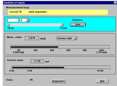
The grey scroll bar becomes active. With this scroll bar you can change the measured value to any value in the range of -10 % ... 110 % and thereby simulate the filling or emptying of the vessel. In the input box of the turquoise window cutout you can enter any percentage value of filling.
