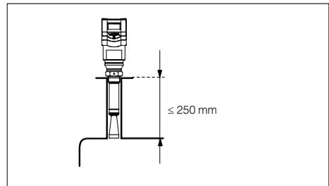
Screw-on antenna with antenna extension on socket piece
