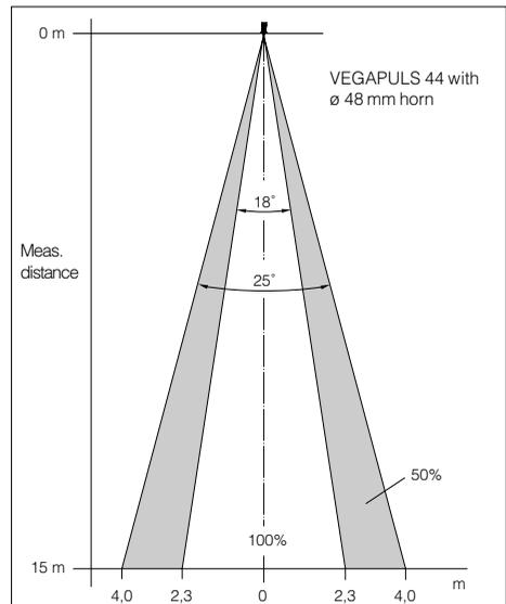
Emission cone of a DN 50 flange antenna
