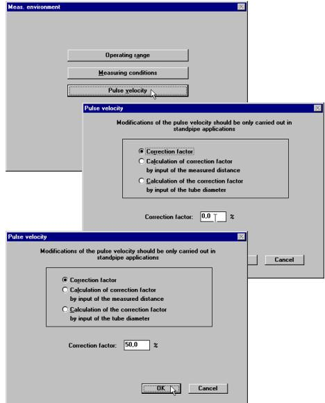
In the menu point "*Pulse velocity*", it is additionally possible to set manually a correction factor for the pulse velocity (light velocity) of the radar signal.
