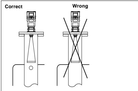
*Pipe antenna: The surge pipe open to the bottom must have a ventilation or equalisation hole on top*
