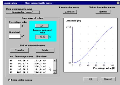
Here the calculated linearisation curve is again outputted. The volume information under "Linearised" now no longer corresponds to the calculated volume of the tank calculation program.
