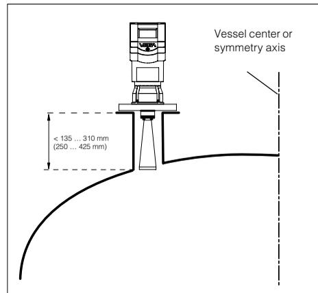
Mounting on a dished vessel top; max. socket length depending on flange size and, if applicable, on the length of the antenna extension (see "3.3 Dimensions").
