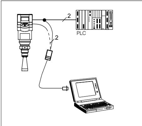
Adjustment with the PC on the 4 ... 20 mA signal and supply cable or directly on the sensor (figure: a two-wire sensor)
