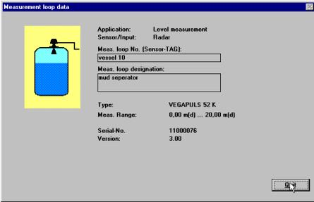
In the window "Measurement loop data", all sensor data are displayed.
