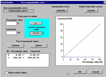
The user-programmable linearisation curve is generated by index markers. Each index marker consists of a value pair. A value pair is composed of a value "Linearised" and a value "Percentage value". "Percentage value" represents the percentage value of level. "Linearised" represents the percentage of vessel volume at a certain percentage value of the level.
