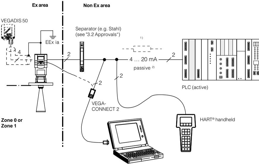
1) If the resistance of the processing systems connected to the 4 ... 20 mA signal output is less than 250 Ω, a resistor must be connected to the connection cable during adjustment to get a loop resistance of 250 Ω. The digital adjustment signal would otherwise be severely damped or short-circuited due to insufficient resistance of the connected processing system. Communication with the PC would not be ensured.
