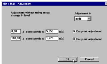
It is convenient and quick to carry out the adjustment without medium, as shown in the example.
