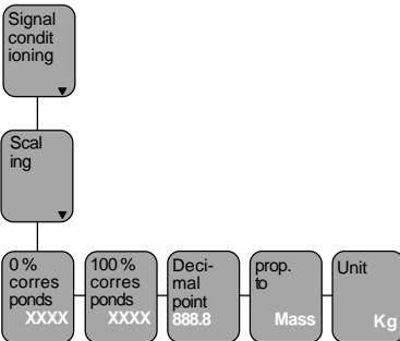
Under the menu item "Conditioning" you assign a product distance at 0 % and at 100 % filling. Then you enter the parameter and the physical unit as well as the decimal point.
