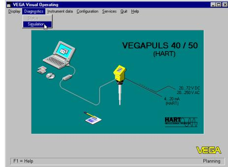
The menu window "Display of measured value" opens. In this menu window you can also set the filling height in the vessel or the signal current and the indication display to any value (simulate measured value).
