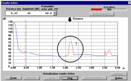
In the next illustration, you see the echo curve after optimum directing of the sensor to the product surface (sensor axis perpendicular to the product surface). The false echo, e.g. caused by a strut, is now reduced by more than 10 dB and will no longer influence the measurement.
