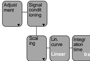
A linear correlation between the percentage value of the product distance and percentage value of the filling volume is preadjusted. With the menu "Lin. curve" you can choose between linear, spherical tank and cylindrical tank. The generation of a customized linearisation curve is only possible with the PC and the adjustment program VVO.
