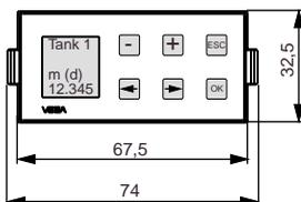
Adjustment module for insertion into series 50 sensors or into the external indicating instrument VEGADIS 50
