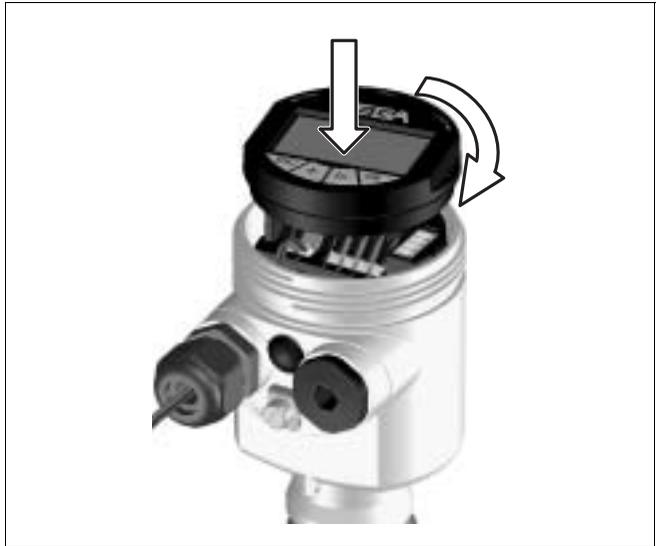
Fig. 29: Installation of PLICSCOM
