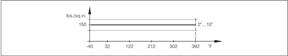
Fig. 44: ANSI flange 150 lbs temperature derating based on °F
