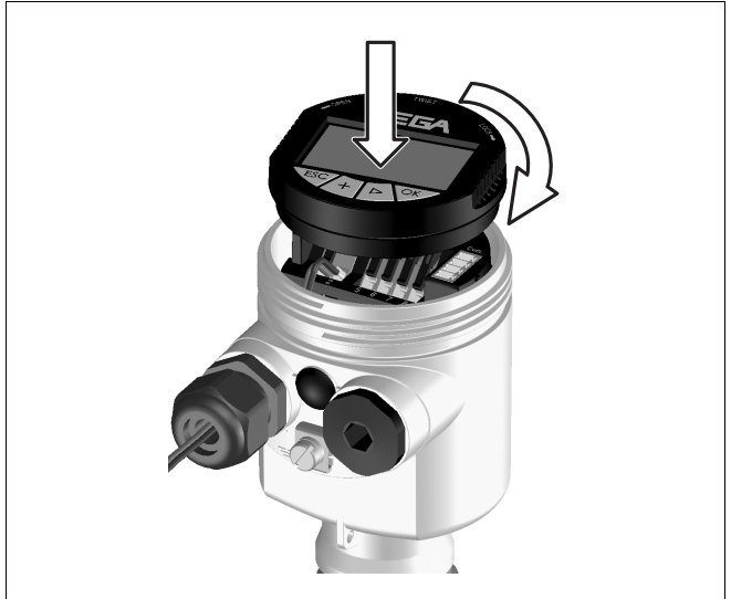
Fig. 24: Installation of PLICSCOM
