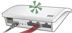
Short-circuit wires (1 second) in the double input which is to control the chosen product(s). It can take up to 1 minute before the light-emitting diode flashes green and the product(s) is/are assigned to the input terminal on the interface.
