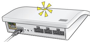
Connect the interface to the mains supply. When the light-emitting diode flashes yellow, the interface is ready for configuration.
