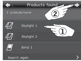
Scroll down the display and choose the product(s) to be assigned to an input ①. The products **must** be of the same type.
