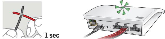
Short-circuit wires (1 second) in the double input which is to control the chosen product(s). The light-emitting diode flashes green.
