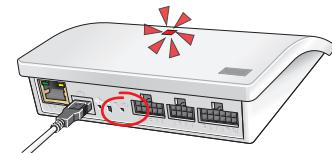
Press the RESET button on the back of the interface for ten seconds with a pointed object until the red light-emitting diode is on. Subsequently, the light-emitting diode turns yellow followed by a red flash.
