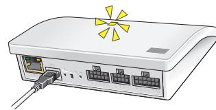
When the light-emitting diode flashes yellow, the interface has been reset. This may take up to 1 min.
