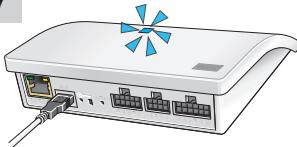
When the blue light-emitting diode is on, the interface is configured as a repeater.
