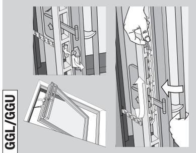
In case of power failure, your centre-pivot window can be closed manually by disengaging the chain on the ventilation flap of the window.
