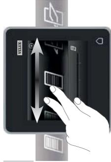
You operate all products by tapping the icons/buttons or by dragging the slider and tapping the bar in the display.
