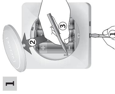
Remove the battery lid by pressing the button with a screw driver as shown in the illustration **1**, **2**.
