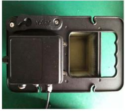
2. turn on the power of WIFI equipment, the equipment include a rechargeable battery, when insert the special charger in the DC socket, it will work by recharge. A full battery can work more than 8 hours. (remark:one time pressing turn it on. more than 3 seconds pressing turn it off, three times continuous pressing reset the system.
