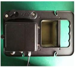
2. turn on the power of WIFI equipment, the equipment include a rechargeable battery, when insert the special charger in the DC socket, it will work by recharge. A full battery can work more than 8 hours. (remark: one time pressing turn it on. more than 3 seconds pressing turn it off, three times continuous pressing reset the
