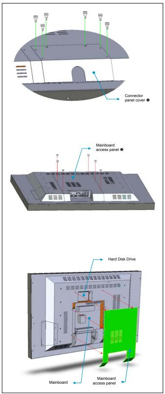
In order to remove the mainboard access panel and gain access to various computer components, the connector panel cover  $(\mathbf{0})$  needs to be removed first.
