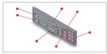
The connector panel is located on the bottom side of the display unit. (Please remove the connector panel cover to access the connector panel)
