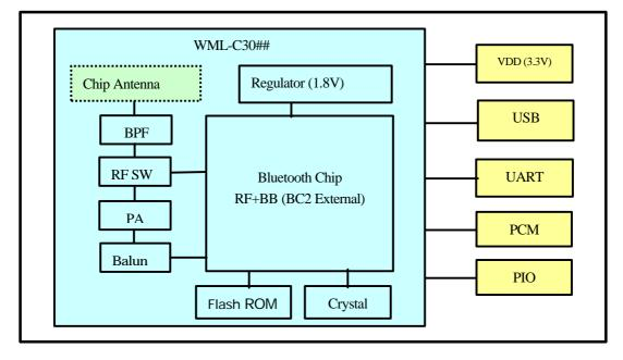
WML-C30## has Bluetooth chip, Flash ROM and Crystal inside. UART/USB HCI interface and PCM interface are used for customer's application. Following figure shows Software Stack for WML-C30## and customer's application as example.
