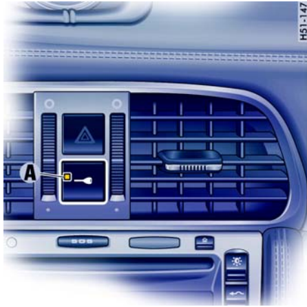
A - Light-emitting diode for alarm system
