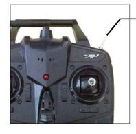
Trainstar Mini comes with pre-installed Gyro to help control flying easily. To turn on the Gyro, switch the knot to upper position(towards you). To turn off the Gyro, switch the knot to lower position(away from you).
