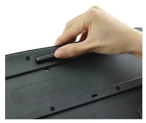
5. Install two AAA batteries into your keyboard following the battery orientation guide in the battery bay.
