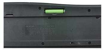
6. Replace the Battery Compartment Cover back onto your keyboard until it securely locks.
