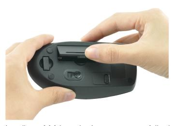
2. Install two AAA batteries into your mouse following the battery orientation guide in the battery bay.
