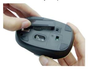
2. Install two AAA batteries into the battery compartment following the orientation guide in the battery bay.
