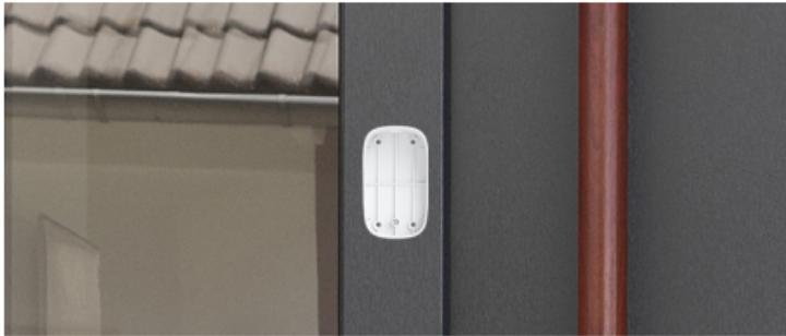
3. Place the weather cover in position on the door frame and hold for 10 second.
