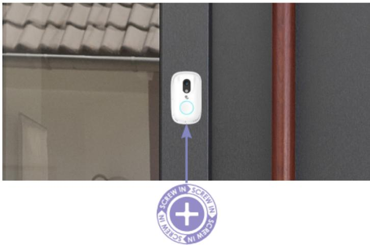
4. Mount the doorbell unit in the cover and screw in the retaining screw.
