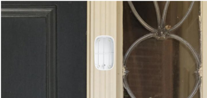
1. Place the rain cover in position, mark and drill mounting screws into place.
