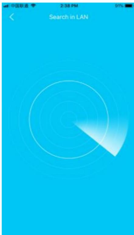
Click on "Search in LAN", you can find all the available cameras in the same router with the smart phone. If added successfully, the camera can be added via the same way by other users (with different account). (**Note:** Cameras that have been added successfully in this account will not be searched again).
