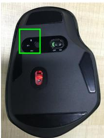
Press the bottom of the mouse to switch the mode button: In 2.4G mode, the indicator light is bright white;
