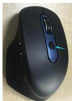
DPI switch button function at the top of the mouse button: DPI speed 5 files: 800-1200-1600-2400-3200 DPI (loop)
