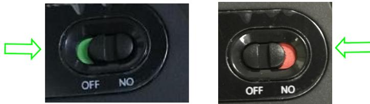
The bottom power control switch, the green flag is ON to turn on the power, and the red flag is OFF to turn off the power.
