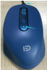
Plug in the USB 5V to the MICRO charging cable. When charging, the red light is always on, and the red light is automatically turned off.
