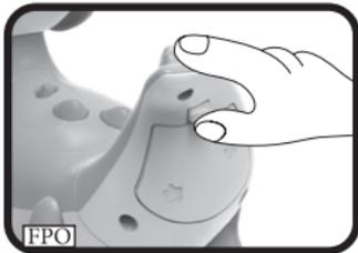
To close the storage, put and align the storage cover with the right place, then press the cover, you will hear a "click" sound.
