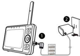
After the parent unit is fully charged, **press and hold** to power on.
