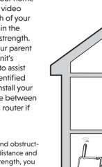
兴 TIP · Depending on surroundings and obstructing factors, such as the effect distance and internal walls have on signal strength, you may experience reduced Wi-Fi signal. To improve the Wi-Fi signal strength, adjust the distance or direction of your parent unit. Check with your parent unit again.
