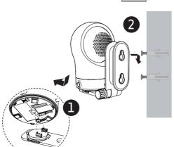
5. You can maximize your camera unit's viewing angles by tilting the wall mount bracket. Hold the camera unit, and then rotate the knob in anticlockwise direction. This will loosen the joint of the wall mount bracket. Tilt your camera unit up or down to adjust to your preferred angle. Then, rotate the knob in clockwise direction to tighten the joint and secure the angle.
