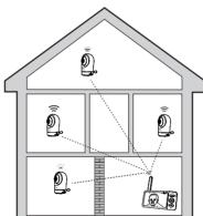
· You may experience reduced signal strength if your parent unit and camera unit are far apart, or there are obstructing factors, such as internal walls, between them. You can set up **Remote mode** to connect via your home Wi-Fi network to improve the connection between your pare camera unit
