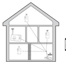
Your parent unit detects the connection signal strength. If you have connected your video monitor with your home Wi-Fi network, your parent unit automatically switches to local or remote mode - the one that has stronger signal strength.
