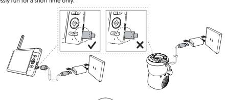
Slide the **ON** switch to power on or off your camera unit.
