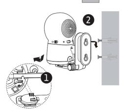
5. You can maximize your camera unit's viewing angles by tilting the wall mount bracket. Hold the camera unit, and then rotate the knob in anticlockwise direction. This will loosen the joint of the wall mount bracket. Tilt your camera unit up or down to adjust to your preferred angle. Then, rotate the knob in clockwise direction to tighten the joint and secure the angle.
