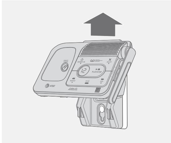
3. Unplug the telephone line cord or the DSL filter from the telephone wall jack. Push the telephone base up and away from the wall-mount bracket to detach it from the wall-mount bracket.
