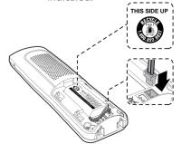
Align the cover flat against the battery compartment, then slide it upwards until it clicks into place.
