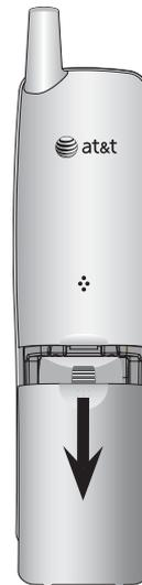
To replace the battery, for optimal performance, charge the handset battery for at least 16 hours before first use. Lift out the old battery and disconnect it from the handset. Follow the instructions on this page to install and charge the new battery.
