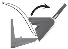
4. Plug the telephone line cord into a telephone wall jack, and plug the power adapter cord into a power outlet not controlled by a wall switch. Route the cords through the channels.
