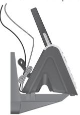
4. Route the telephone line cord through the bracket hole and plug it into the wall jack or a DSL filter (if required). Align the holes on the bracket with the standard wall plate and slide the bracket downward on the mounting studs until the telephone is secure. Plug the power adapter into a power outlet not controlled by a wall switch.
