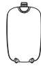
Battery compartment cover (1 for CS6114/CS6114 B/ CS6114-11/CS6114-11 B) (2 for CS6114-2/CS6114-2 B/ CS6114-21/CS6114-21 B)
