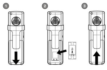
CAUTION: Risk of explosion if battery is replaced by an incorrect type Dispose of used batteries according to the instructions
