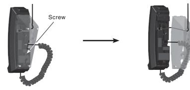
4. Rotate the mounting bracket. Insert the tabs of the mounting bracket into the lower grooves of charging base. Then tighten the screw to affix the mounting bracket.
