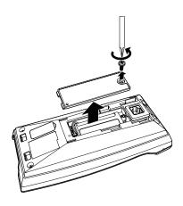
2. Remove the used battery from the comparment. Plug the new battery connector securely into the socket inside the base battery compartment. Place the battery with the label **THIS SIDE UP** facing up and the wires inside the battery compartment.
