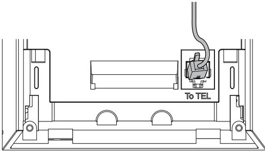
2. Align the grooves of the base stand with the telephone base. Slide the base stand up to secure it.
