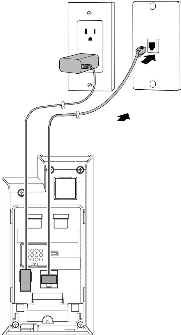
2. When the telephone base has been initially installed, make sure the power adapter is securely plugged into an outlet not controlled by a wall switch, and the Ethernet cable is plugged into the network wall jack.
