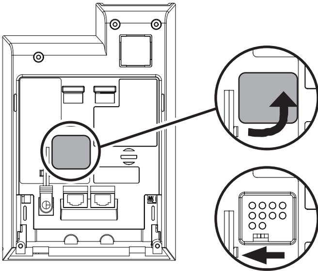
2. Slide the base power switch to the off position.
