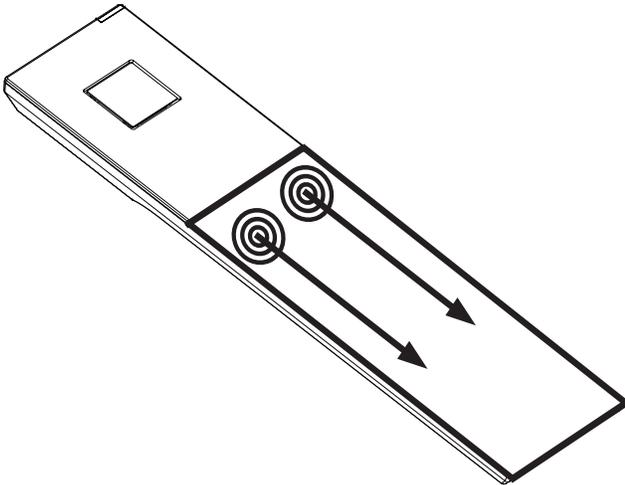
3. Lift the battery cover off the handset.
