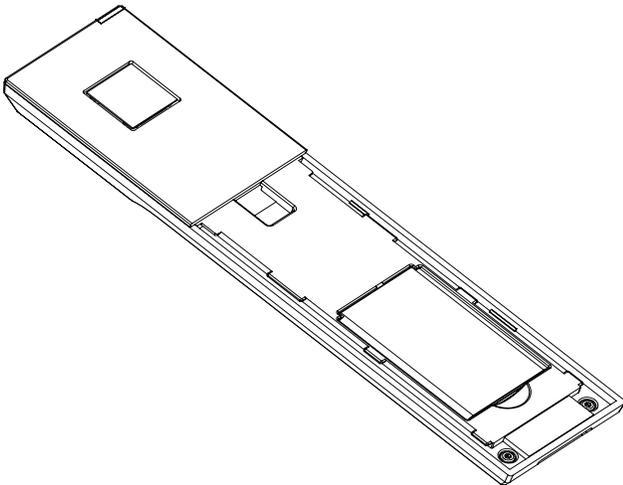
4. If you are replacing the battery: Place your thumb in the slot below the battery, and lift the battery out of the handset battery compartment.
