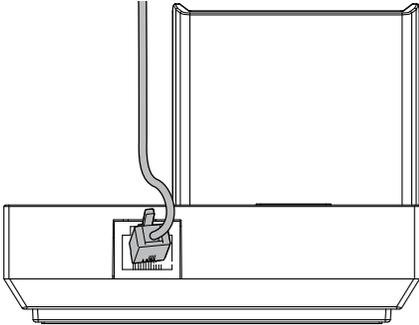
2. Plug the other end of the telephone line cord to the telephone wall jack and the power cord connector to the power adapter. Plug the power adapter to a wall power outlet.
