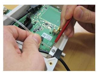
4. Pull the pressure tube out of the tube fitting piece
