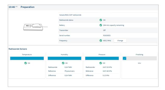
If the ground check device you are using to prepare RS41-SGP(E) does not include a pressure sensor, type the reference pressure and select **Apply**. If the pressure sensor is included, the value is obtained automatically.
