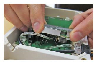
3. Push the barometer module in place.
