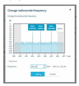
3. To set the new frequency, use the arrow buttons or select the correct frequency in the radio spectrum, and select **Save**.
