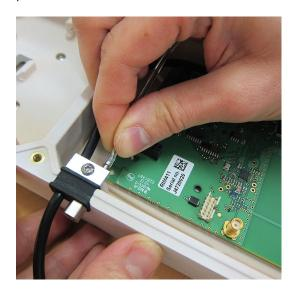
2. Check the connector positions on the barometer module and place the barometer module in the correct position in RI41-B.
