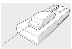
The radiosonde is automatically switched on when placed on the ground check device. The sounding software automatically detects the radiosonde and begins the preparations.
