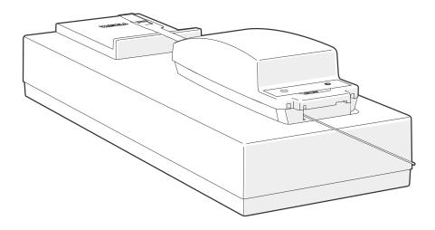
Vaisala Ground Check Device RI41 is available in 2 models: RI41, and the similar RI41-B, which is equipped with a barometer module. The RI41-B is used together with RS41 radiosondes with in-built pressure sensors, such as the RS41-SGP. During the ground preparation procedure, the reference barometer in the RI41-B is used to adjust the measurement of the in-built pressure sensor in the radiosonde.
