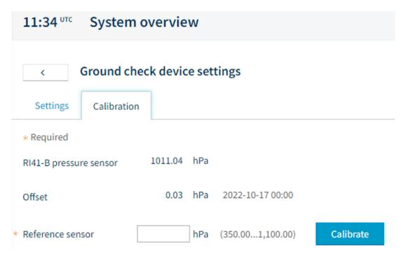
The system shows you the current barometer pressure reading, offset value, and date of the last calibration.
