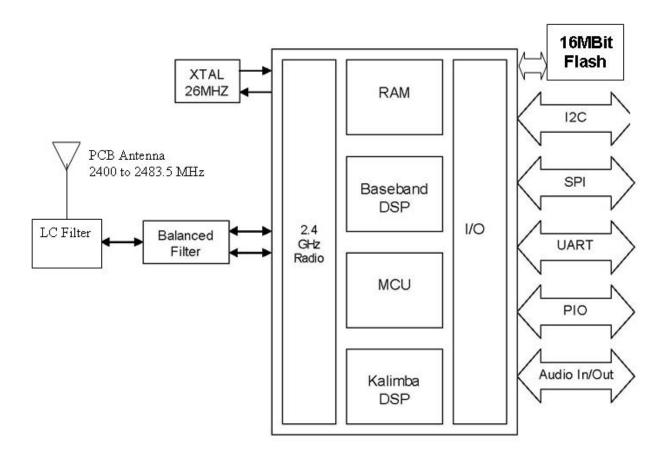
IBT05(C) is a Class 2 Bluetooth sub-system using BlueCore5 –Multimedia Ext Flash chipset from leading Bluetooth chipset supplier Cambridge Silicon Radio. .It interfaces to a 8/16 MBit parallel Flash. The software stack running on the BlueCore5 MM Ext chipset is fully compliant to Bluetooth Specification v2.1 + EDR. iBT04(5) also has necessary balun and bandpass filters to interface with a build-in PCB antenna, which forms a very cost effective radio subsystem.
