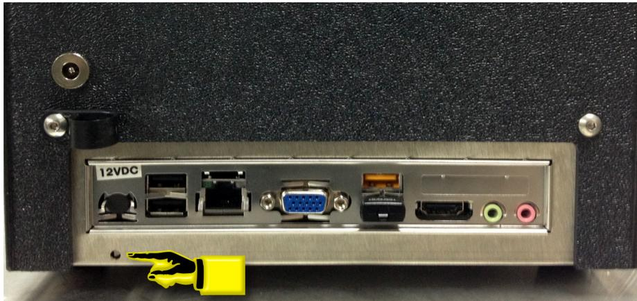
The reset button is located directly below the connector for the power cord and is accessible via the small hole. Using a small tool or a paper clip, insert it into the hole and toggle the switch.
